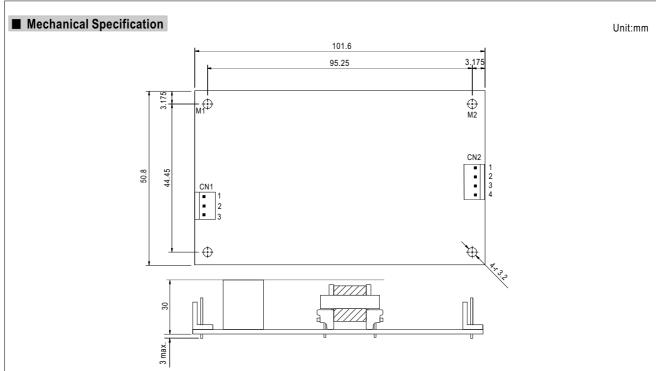
AC Input Connector (CN1): JST B3P-VH-B or equivalent
